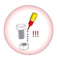
All screws, nuts and sleeves must be secured with Loctite (except stop nuts)
