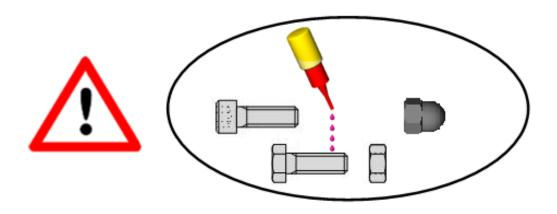
glue all screws, nuts and sleeves with loctite.
