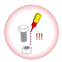
Glue all screw's, nuts and sleeves with loctite. (not les than 5 drops!) (except for lock nut)
