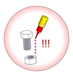
Glue all screws, nuts and sleeves with loctite. (not less than 5 drops!) (except for lock nut)
