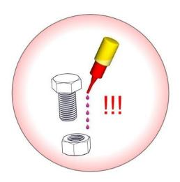
Glue all screws, nuts and sleeves with loctite. (not less than 5 drops!)(except for Nyloc nuts)
