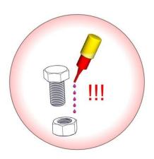
All screws, nuts and bushes (e.g. Torx-bushes) must be secured by Loctite! (stop screw nuts excepted
