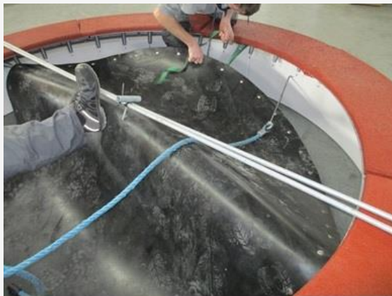
Fit tensioning strap 90 ° offset and opposite spring Hook.
